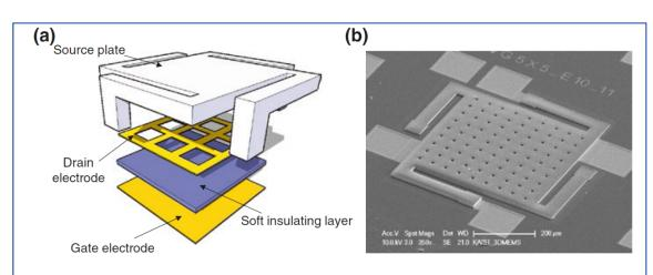
Fig. 11 a Schematic illustration and b SEM image of the stacked electrode MEMS switch with a soft insulating layer [33]
