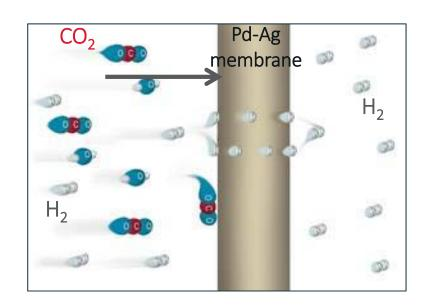
For  $Pd_{0.75}Ag_{0.25}$  alloy, the permeability of  $H_2$  is given by the following design equation:
