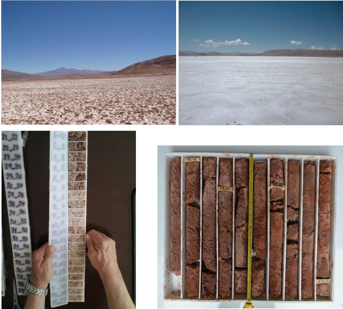
Figure A2 Top: Surface examples of the Salar de Pozuelos. Hard and rough salt crust from the central part of the salar (left) and smooth salt crust from the margin (right). Bottom: Halite and red clay to fine sandstones from the drill core.
