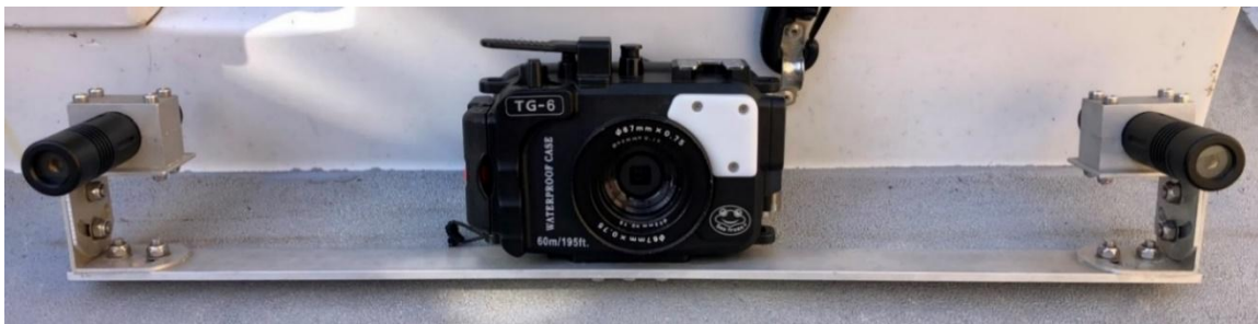
Supplementary Figure 1 Custom-made paired-laser photogrammetry rig consisting of a steel bracket mounting two green lasers (OceanCo Shark Lasers) 50 cm apart, aligned in parallel with an underwater camera (Olympus Tough TG-6 in Sea Frogs waterproof housing)
