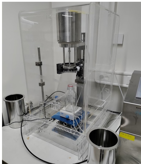
Fig. S1: Axenic bead production setup with a plexiglass box around the Nisco encapsulator.
