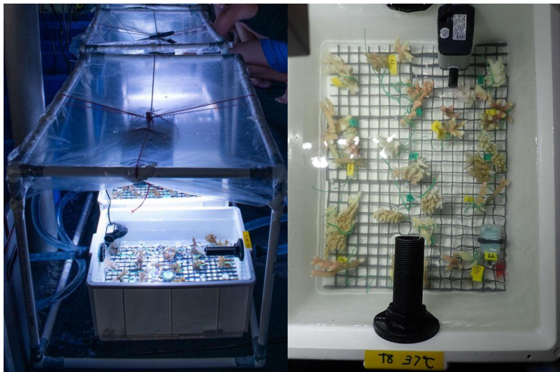
Fig. S1 Images of the experimental setup. Portable experimental temperature tanks with flow-through system set up on the boat deck (left-side). An example of coral fragments (mostly bleached) in the 37°C tank (right-side) along with the water circulation powerhead (top right corner) and hobo temperature logger (bottom right corner). Note, there are also Acropora millepora fragments in this photo that were not part of this manuscript.
