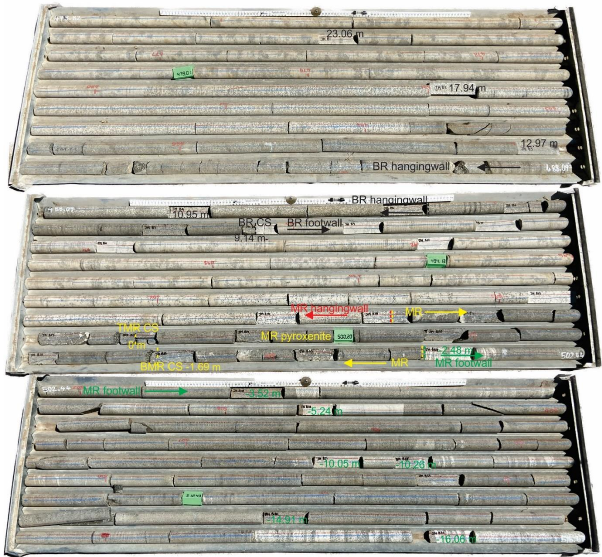
Figure A.1: Photographs of the core boxes hosting the Bastard and Merensky reefs. BR = Bastard Reef, BR CS = Bastard Reef chromitite stringer, MR = Merensky Reef, TMR CS = Top Merensky Reef chromitite stringer, BMR CS = Bottom Merensky Reef chromitite stringer.
