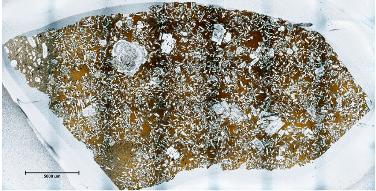
Figure S1b. Small enclave C1163. Fine-grained material in the upper and lower left is host rock. Note oversized zoned plagioclase crystal in upper left that appears to be incorporated from host (same image in cross-polarized light shown in Fig. S5). Vertical stripes in image are an artefact of the stitching process.
