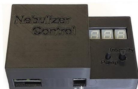
Ports for the atomizers
