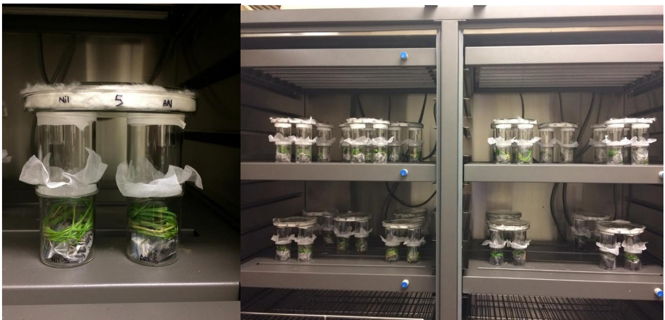
Figure: Glass still-air olfactometer used to assess Argentine stem weevil ( Listronotus bonariensis ) olfactory responses to perennial ryegrass
