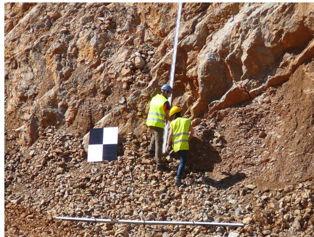
Figure ESM01-6. Detail of the targets and surveying staffs deployed over the scene for georeferencing.
