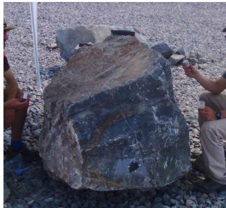
Figure ESM01-4. Test 3 site, measuring the sound velocity across a block with a Pundit sclerometer and two opposite geophones.
