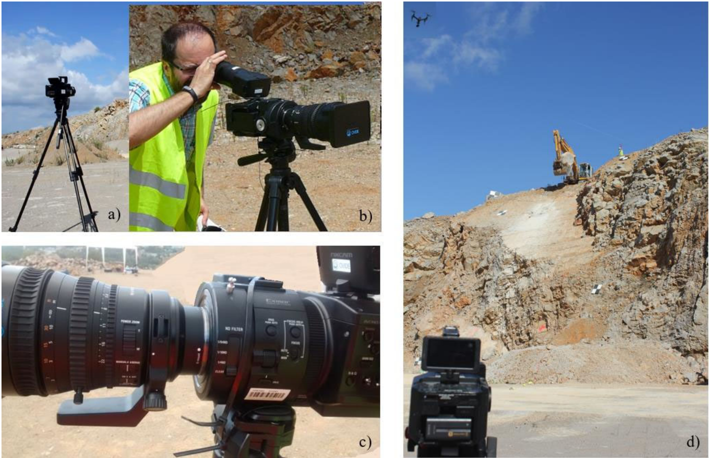
Figure ESM02-2. High-Speed video camera, Sony NEX FS700R. a, b) The camera over its tripod. c) Camera close-up. d) During a block release (Test 4 site). Note the drone flying over the esplanade.
