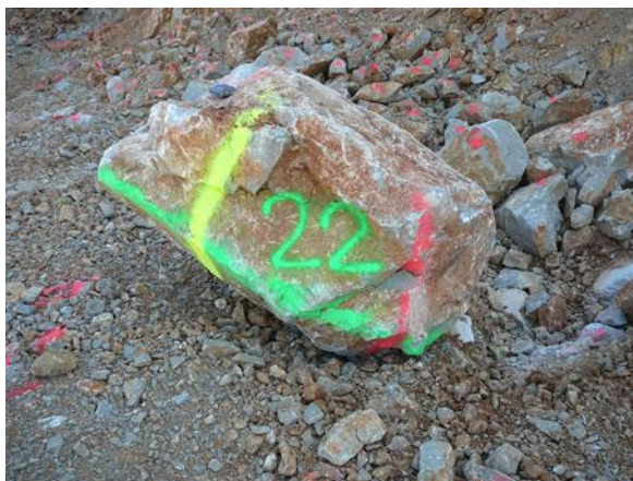
Figure ESM02-3: big fragment of block #22 (Test 1) surrounded by small fractions. The pink dots in some fragments around the big one intended to avoid double counting.
