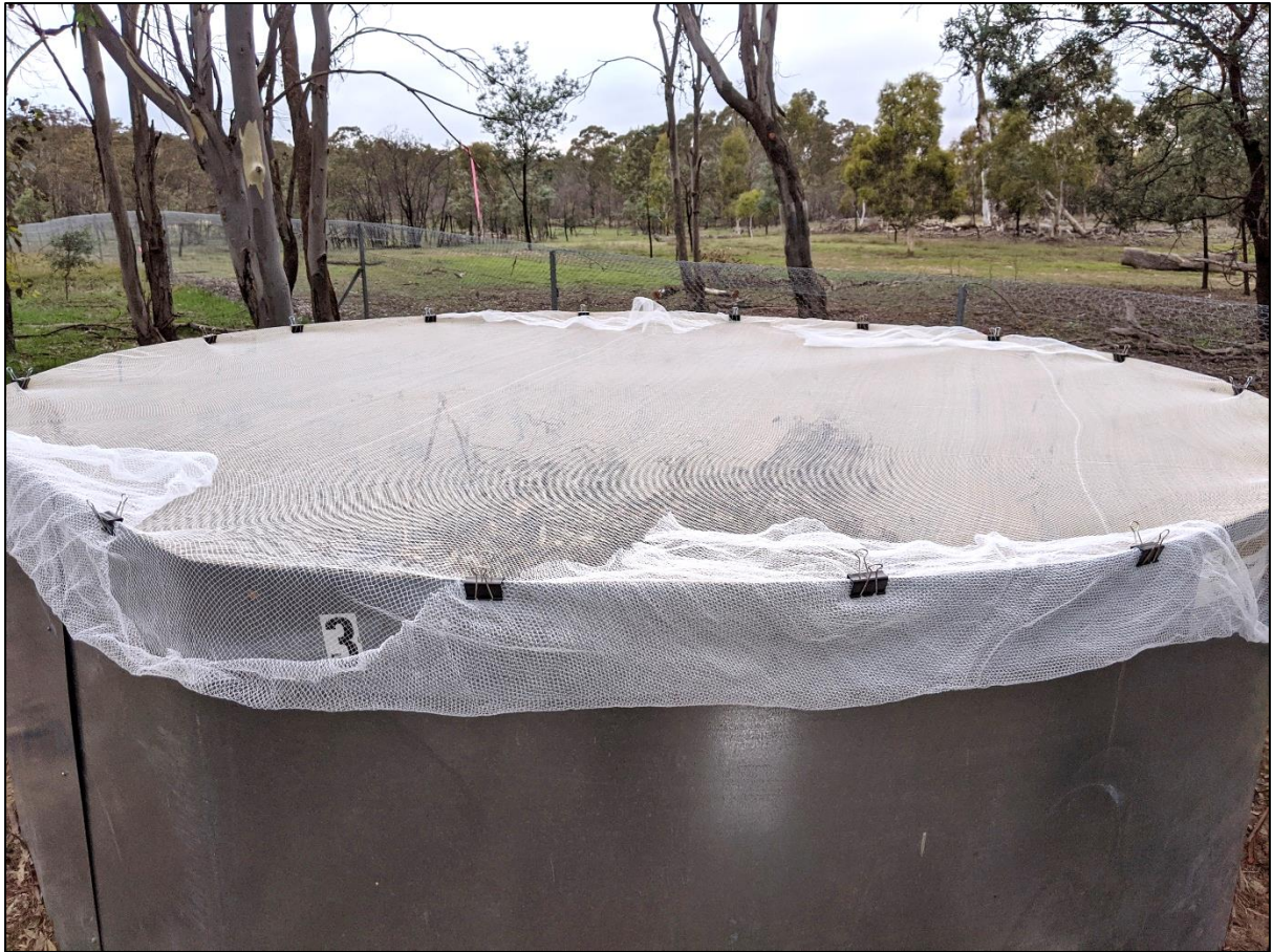
Fig. 2 Ring-tanks were made from sheet metal ( \sim 1.2 mm thick), dug \sim 100 mm into the ground and internally supported by metal stakes secured to the walls. The ring-tank was accessible through a join held together by a bolt at the top and bottom (above ground level). All other joins were held together with screws. Two mouse holes and single large hole each had a removeable door made from 0.5 mm sheet aluminium held on with multiple bolts. Leafy branches and mouse houses were added to the ring-tanks for shelter. For Trial 2 only, we covered ring-tanks with fine fruit-netting held taut with fold-back clips. These clips were not strong enough to stop possums from jumping in. We suggest the use of screws to hook the netting over the walls, instead of fold-back clips. Refer to the main text for an illustration with approximate measurements
