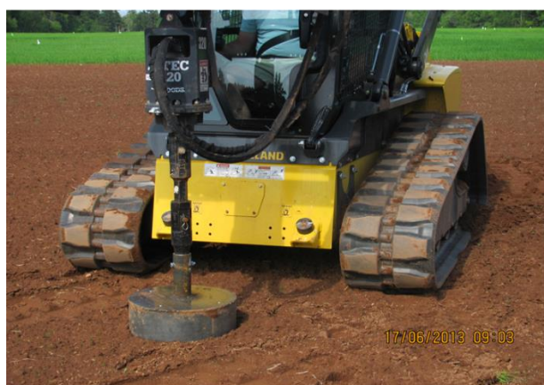
Figure S1. Container (open cylinder) installation using a prototype cookie cutter saw blade cut created specifically for this project
