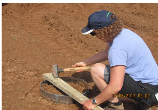
Figure S1. Container (open cylinder) installation using a prototype cookie cutter saw blade cut created specifically for this project
