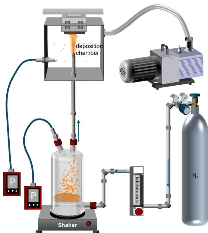
Fig. S1: Schematic illustration of the powder aerosol deposition (PAD) setup without the use of an ejector–separator unit and without an inertial separator having a collecting tube
