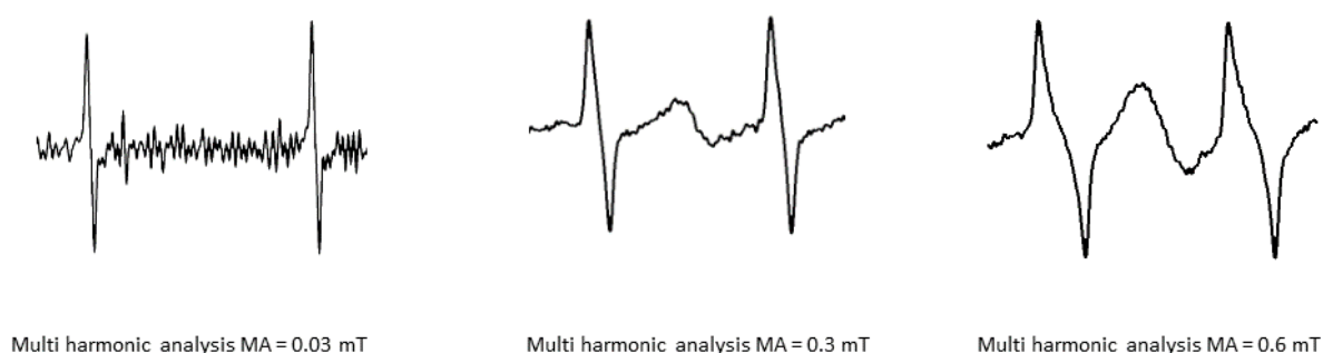
Fig. S1: Multi-harmonic reconstruction of the signal recorded on a melanin phantom. The EPR spectrum contains signals coming from melanin (center) and the doublet of ^{15}\text{N} -PDT (low and high field signals) used as a reference. The analysis allows the reconstruction for a given modulation amplitude. At high modulation amplitude, the signal of melanin (that presents a large EPR linewidth, around 0.5-0.6 mT) is clearly visible without distortion while the ^{15}\text{N} -PDT appears distorted. Using a reconstruction with low modulation amplitude, the signal of melanin is almost invisible while the ^{15}\text{N} -PDT signal is not distorted with its inherent narrow linewidth (0.03 mT).
