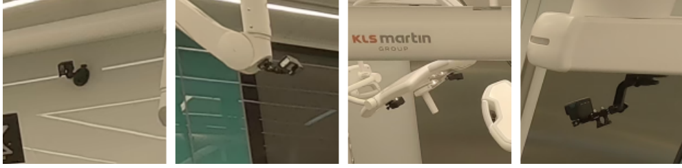
Figure 2: From left to right: far-field camera mounted on the wall, followed by three near-field cameras mounted on different sections of a surgical lamp within the operating room.
