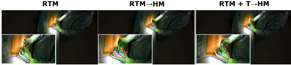
Figure 5: Qualitative comparison of 3D hand poses estimated using baseline methods and our approach (shown reprojected onto input images). From left to right: RTM Whole-Body, RTM \rightarrow HM, and our method combining intermittent RTM, hand tracking, and HM. The first detects both hands but with coarse joints, the second misses one hand and mislocalizes joints, while ours accurately detects and localizes both hands.
