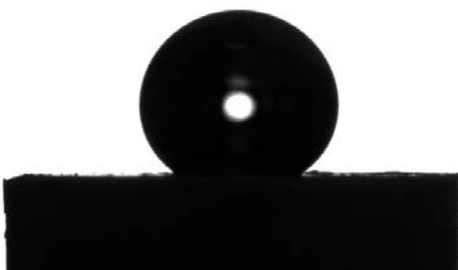
Figure S8. Water droplet on the tablet of octyl-functionalised silica nanoparticle (trimethoxy(octyl)silane : nanoparticle = 200 \mu\text{L} \cdot \text{g}^{-1} )
