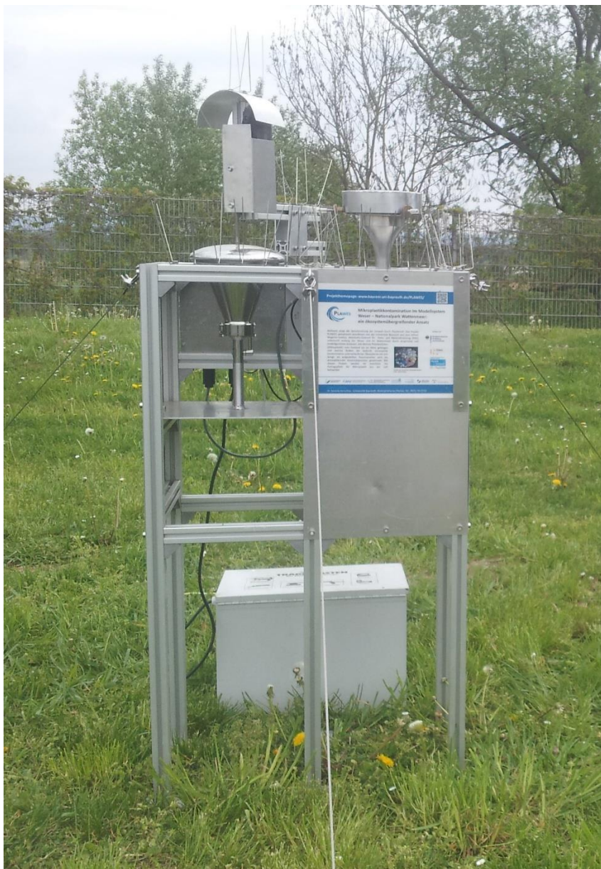
Figure S2: Wet and dry atmospheric deposition collector.
