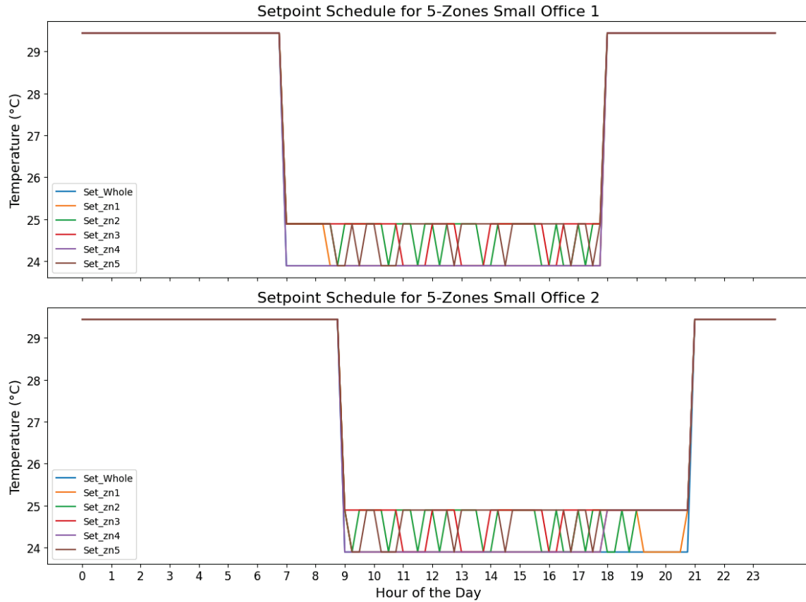
Figure 7. Temperature setpoints for Small Office
