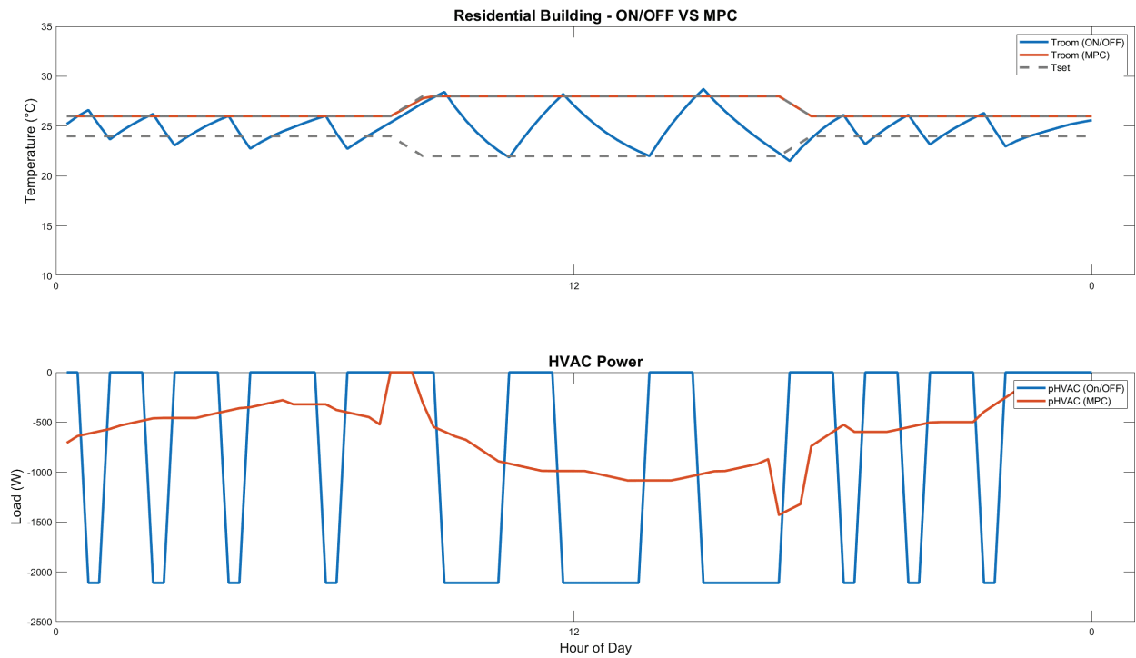
Figure 9. Single-zone residential building RC model MPC vs. ON/OFF control
