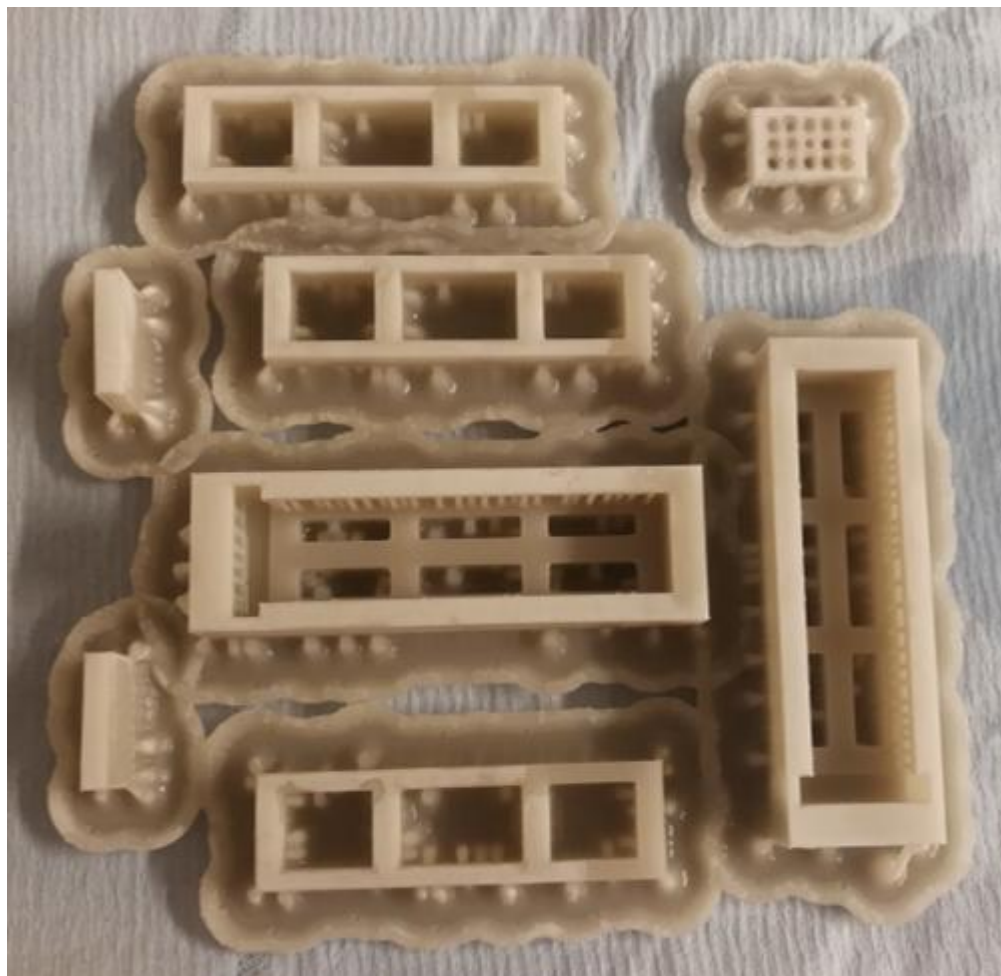
Figure S1 The 3D printed cage component precursors. After trimming and polishing, the cage components were baked to remove the wax composition in the resin and partially anneal the \text{SiO}_2 to get an integrated part (1100 °C resistance).
