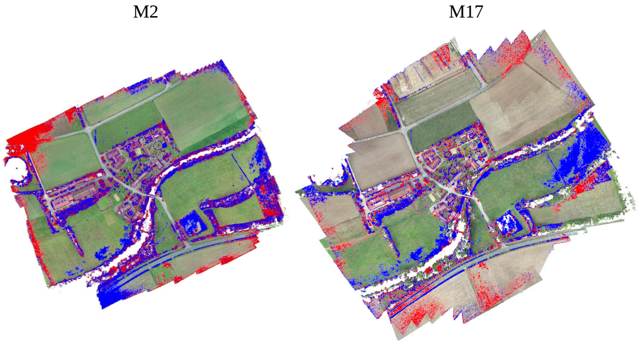
Fig. 9 Areas with detected changes between survey 1 and 2 of M2 and M17 in the Laufer Muehle area ( |d_{M3C2}| \geq 0.25 m ; red: elevation increase in survey 2; blue: elevation decrease in survey 2)
