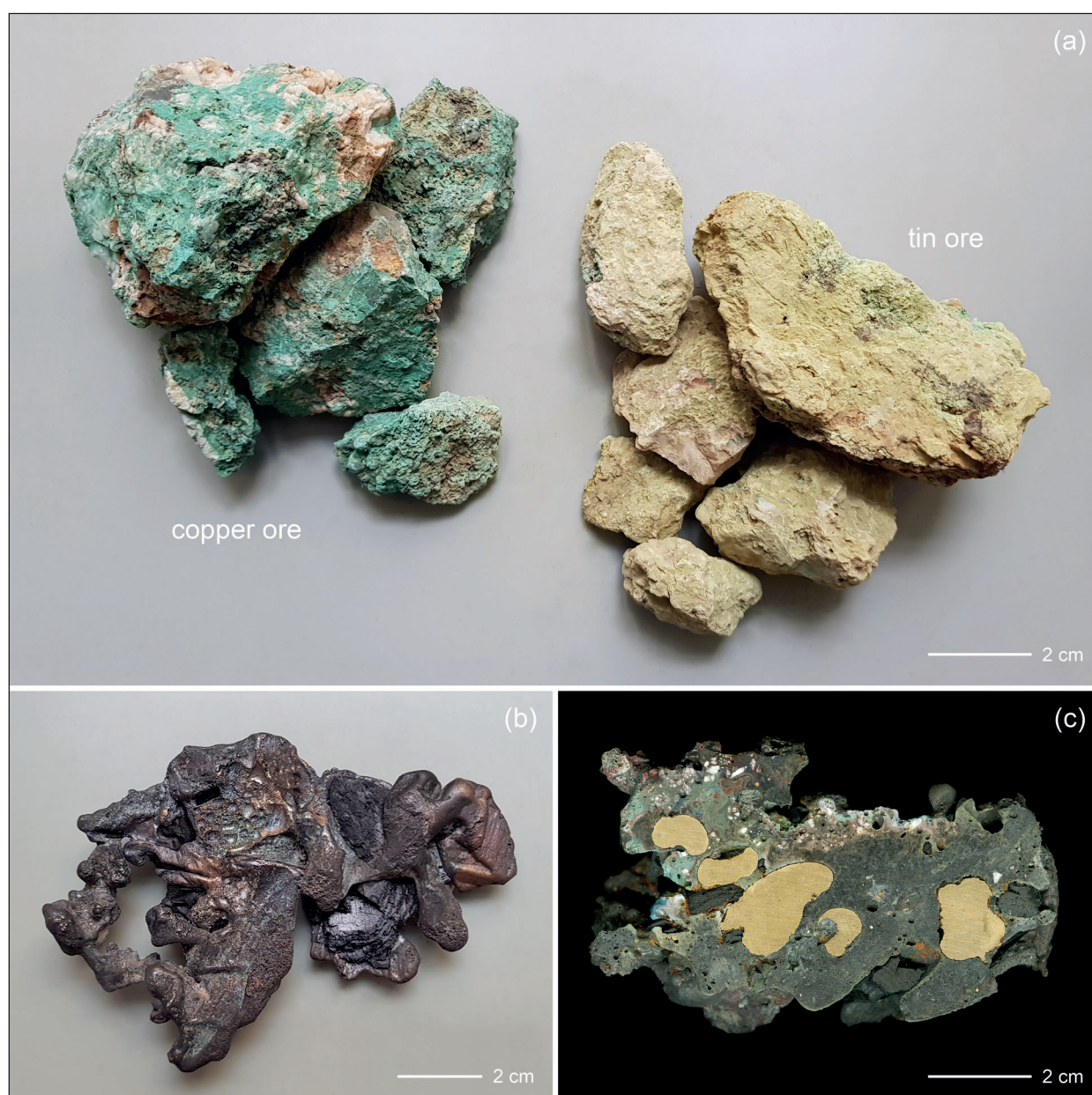
Fig. 2 Copper and tin ores from Mušiston that have been used for the smelting experiments (a) and bronze lump (b) and bronze slag (c) obtained from experiment 2 (photos: D Berger).
