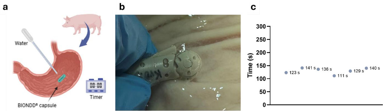
Fig. S1. (a) Illustration of the ex vivo pig stomach model. Pig stomachs acquired directly from the slaughterhouse are cleaned and cut open. The stomach tissue is laid out flat, and a BIONDD® capsule is placed on the inside tissue of the stomach. Water is added dropwise, and the time it takes for the device to actuate (i.e., the capsule to dissolve) is noted. Following device actuation, the spike insertion is visually inspected and photographed. Created in BioRender. Mertz, N. (2026) https://BioRender.com/b26fyf7 . The study was carried out under a permit for handling animal byproducts provided by the Ministry of Food, Agriculture and Fisheries of Denmark (license: DK-123-oth-1425482). (b) BIONDD® prototype device after actuation with spike inserted into ex vivo pig stomach tissue. (c) Individual actuation times recorded for the BIONDD® prototype device (n = 6) using the ex vivo pig stomach model. The average actuation time was 130 \pm 12 s. Insertion of the spike into the ex vivo pig tissue after device actuation was observed for all of the 6 BIONDD® devices.
