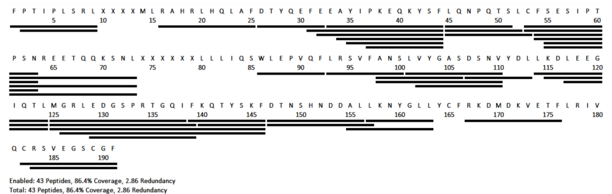
Supplementary Figure 2. rhGH peptide maps generated by MS E (a) HDMS E (b) and UDMS E (c) modes of acquisition.
