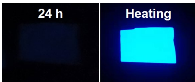
Fig. S24. PeL photographs of the GC:Eu after 24 h at room temperature (left) and heated at 150 °C (right). The PeL intensity after 24 h is quite weak, but it can be brightening again through heating, indicating that the deep traps with a slow electron releasing rate can capture many electrons as well.
