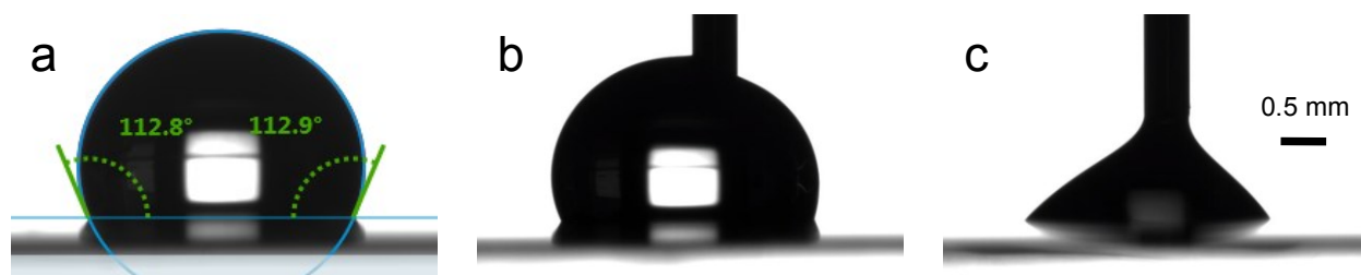
Figure S5 Water contact angles. (a) Static water contact angle. (b) Advancing contact angle. (c) Receding contact angle. To obtain the dynamic contact angle, 5 \mu\text{L} of deionized water was placed on the surface, followed by expanding and shrinking of deionized water at a rate of 0.1 mL/min via the needle of the syringe. The process was recorded by a camera. Advancing contact angles were obtained from the snap-shot during expanding process while receding contact angles were obtained from the one during the shrinking process.
