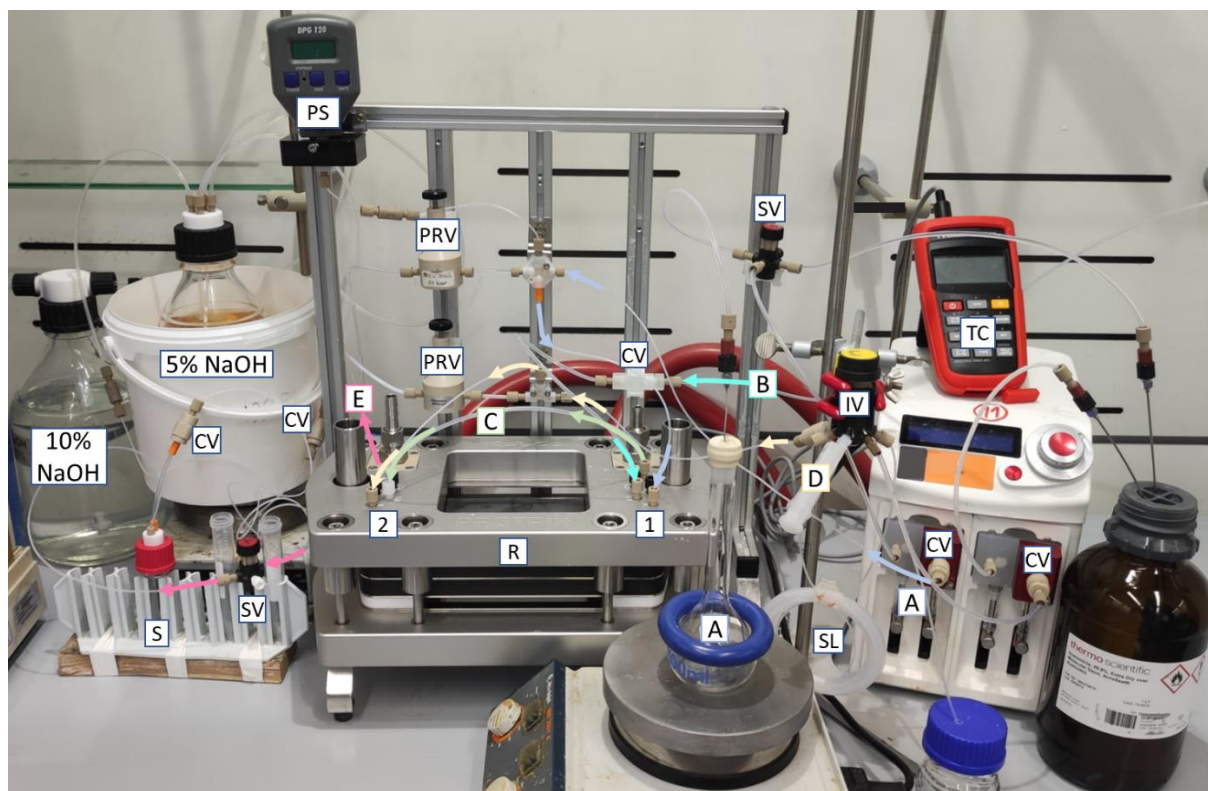
Figure S9. Image of the continuous flow set-up for the telescoped diCINFPy 2 generation and fluorination of enamine 3 . CV: Check Valve; SV: Switching Valve; S: Sampling; PS: Pressure Sensor; PRV: Pressure Relief Valve; IV: Injection Valve; SL: Sample Loop; TC: Temperature Control for the Huber thermostat (not shown); A: DCP-BF 3 complex 1 feed (0.1 M), B: 10% F 2 /N 2 feed, C: diCINFPy 2 outlet connected to second reactor volume for the enamine fluorination, D: enamine 3 feed, E: reaction mixture outlet. R: Protrix SiC reactor using 2 modules; 1: Reactor volume 1 for diCINFPy 2 generation; 2: Reactor volume 2 for the fluorination of enamine 3 with in-situ generated diCINFPy 2 .
