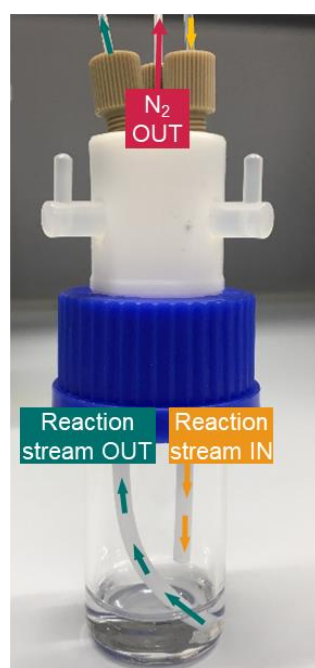
Figure S2. Self-made gravity-based gas/liquid separator.
