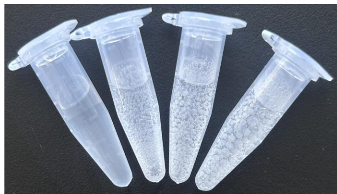
Fig.S23 O 2 bubbles produced by different volumes of DNA-Au/Pt catalyzed H 2 O 2 (500mM, 1mL) solution for 5 min (from left to right: 0,10, 20, 40μL)
