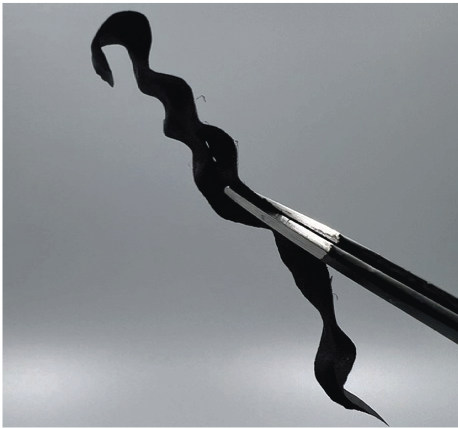
Figure S5: Photographs of a pure PVA/MWCNT composite film after exposure to elevated conditions ( \sim 50^\circ\text{C} and 70% RH), showing visible warping and shrinkage.
