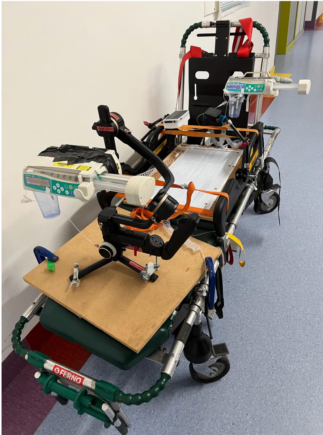
Set up of phase 3: One pump mounted on a gimbal, the other secured to the trolley with a clamp, pointing in the same direction
