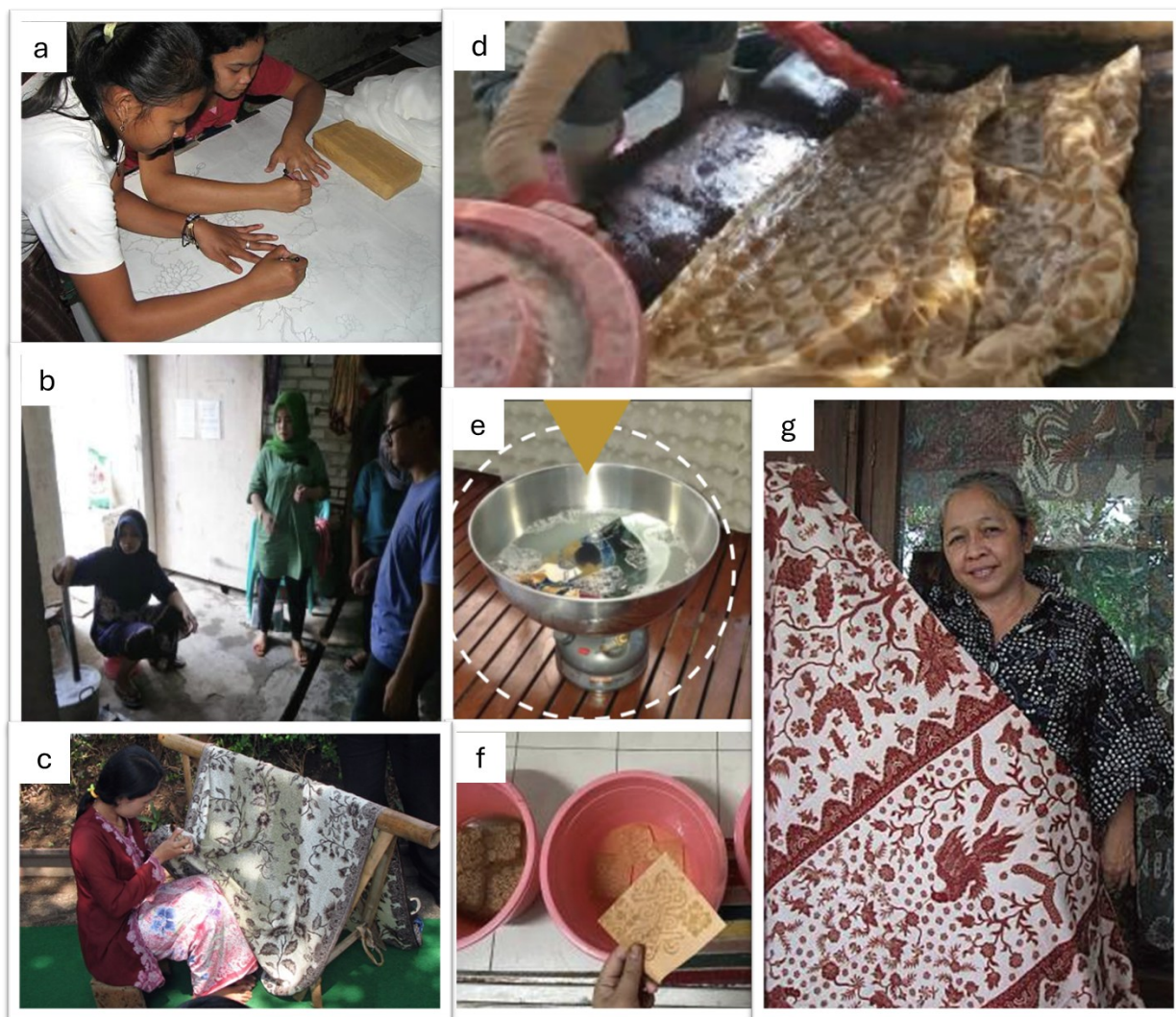
Fig. S2 Batik Production Process: (a) designing, (b) mordanting, (c) waxing, (d) dyeing, (e) wax removal, (f) fixation, and (g) drying [2–5].
