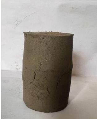
Fig. 6: UCS failure pattern of peat soil For a 28-day curing period
