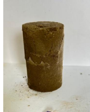
Fig. 7: UCS failure pattern of S+15C for 28-day curing period
