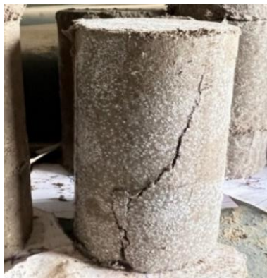
Fig. 13a: UCS failure pattern for S+15C+12RHA for a 28-day curing period.
