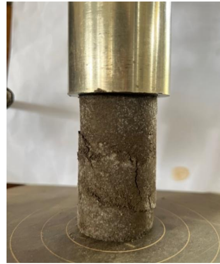
Fig. 11: UCS pattern of S+12RHA for The curing period lasts for 28 days.
