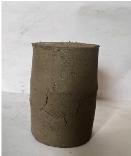
Fig. 10: UCS failure pattern of Peat soil for a 28-day curing period
