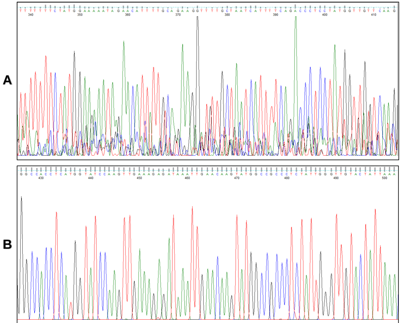
Supplemental Figure 2. Sample sequencing chromatogram traces. (A) An example of poor quality sequences from the Eh_07 rbcL amplicons following the sequence chromatogram analysis; it is characterized by too much baseline noises and peaks that are difficult or impossible to call. (B) An example of good quality sequence from Eh_03 rbcL amplicons following the sequence chromatogram analysis; it is characterized by the absence of baseline noises and easy to call peaks (Q value > 20).
