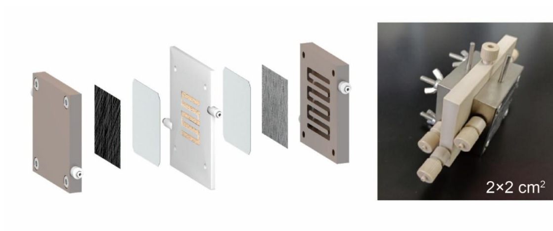
Figure S22. Schematic illustration and the photograph of a PSE reactor.
