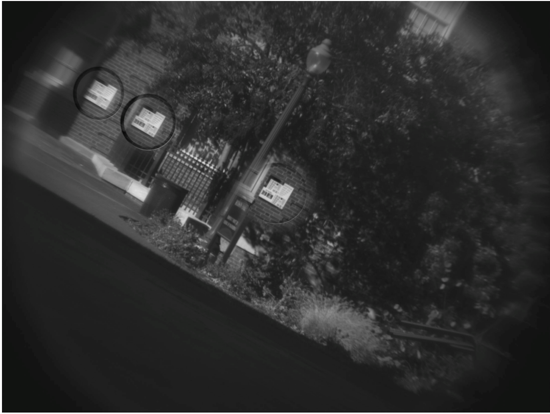
Supplementary Figure 4.5. Superposition of three separate images, showing the field locations in camera 017 for the resolution charts shown in Supplementary Figure 4.1. The target was stationary on the building while the camera was rotated for the three field locations.
