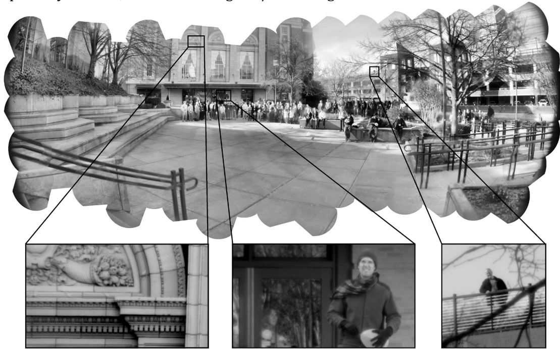
Supplementary Figure 4.3. The Carolina Theatre in Durham, North Carolina. Top shows a full, stitched image from the AWARE-2 camera, featuring 98 microcameras. The bottom insets show zoomed in regions of the image at 11.5x relative to the full image. Each camera has an optimal exposure, dramatically increasing the usefulness of the camera in high-contrast settings.
