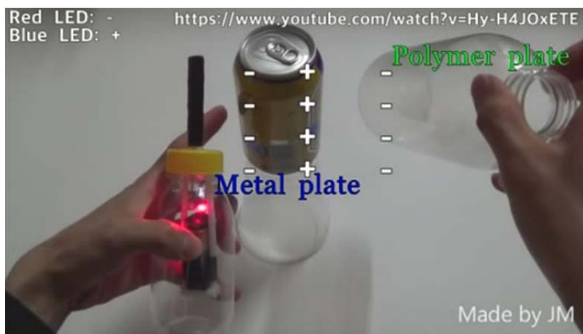
Movie 1 | The charges separated in the metal plate by the electrostatic field of the charged polymer.
