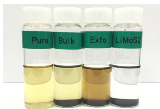
Supplementary Figure 5. Comparison in reducing power of 2H and 1T' phase with \text{Na}_2\text{PtCl}_6 . From left to right: pristine \text{Na}_2\text{PtCl}_6 \cdot 6\text{H}_2\text{O} solution (17.6 mg in THF), with 50 mg bulk \text{MoS}_2 , exfoliated \text{MoS}_2 and \text{Li}_x\text{MoS}_2 after heating at 80 °C for 2 days. Exfoliated \text{MoS}_2 nanosheets only show weak reducing power due to the loss of 1T'-phase after water exfoliation.
