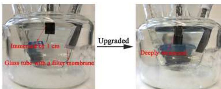
Figure R22 | The three-electrode system for electrocatalytic HER stability tests.
