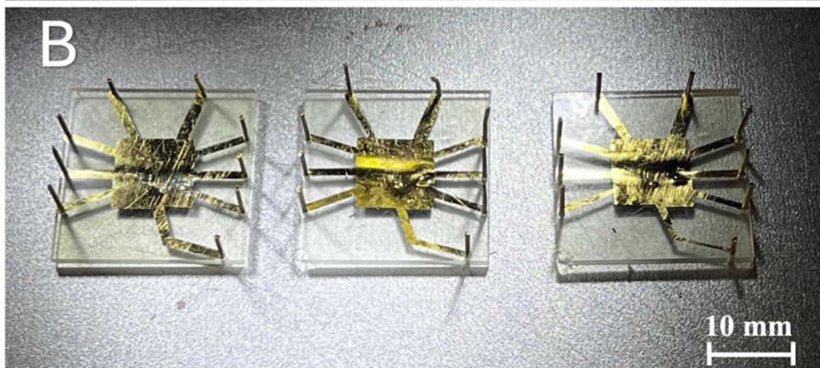
Supplementary Figure 1: A) Optical image of the 5x5mm 2 MEA configuration with a total conductive area of ~13.04mm 2 . B) Optical image of the 5x5mm 2 MEA configuration with a total conductive area of ~19.71mm 2 .
