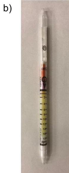
Figure S25 The photo of a gas detection tube for detection of HBr. a) Reaction scheme of this experiment. b) A result of the gas detection. A microtube with 19.8 mg ( 1.7 \times 10^{-4} mol) of pure compound 4 and 35.9 mg ( 2.1 \times 10^{-4} mol) of hydrobromic acid (49%) was put into the 1000 mL beaker overnight in closed system. After the reaction, we covered the mouth of the beaker with oil-based clay and glass plate, and insert the detector tube. This gas detector tube turns to bluish purple from yellow, if HBr gas was detected. In this investigation, we sucked the gas with gas detector tube (No.136LA) in once, the scale of the tube showed 18 ppm. Generally, when using this detector tube, the basic number of suction is twice. Therefore, we multiplied 2 to the scale. From the calculation, the concentration of the MeBr gas was 34 ppm.
