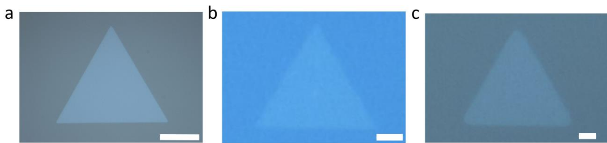
Supplementary Figure 12 | Optical micrographs of as grown monolayers. Optical micrographs of as-grown WSe 2 monolayers on (a) fused silica, (b) aluminum nitride, (c) sapphire. Scale bars are 20 \mu\text{m} , 2 \mu\text{m} , and 2 \mu\text{m} respectively.
