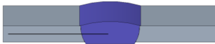
Figure 2: Center line of vertical transversal cross-section for microhardness testing
