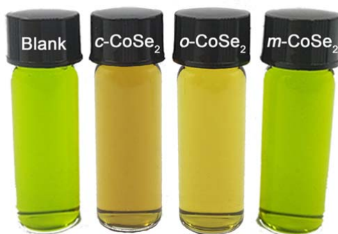
Figure R2. Colorimetric comparison of the cycled electrolytes added in sodium acetate and nitroso-R salt solution. No color change was seen for m-CoSe 2 , indicating its marked structural stability in acidic electrolyte. Nitroso-R salt was used as the color indicator.
