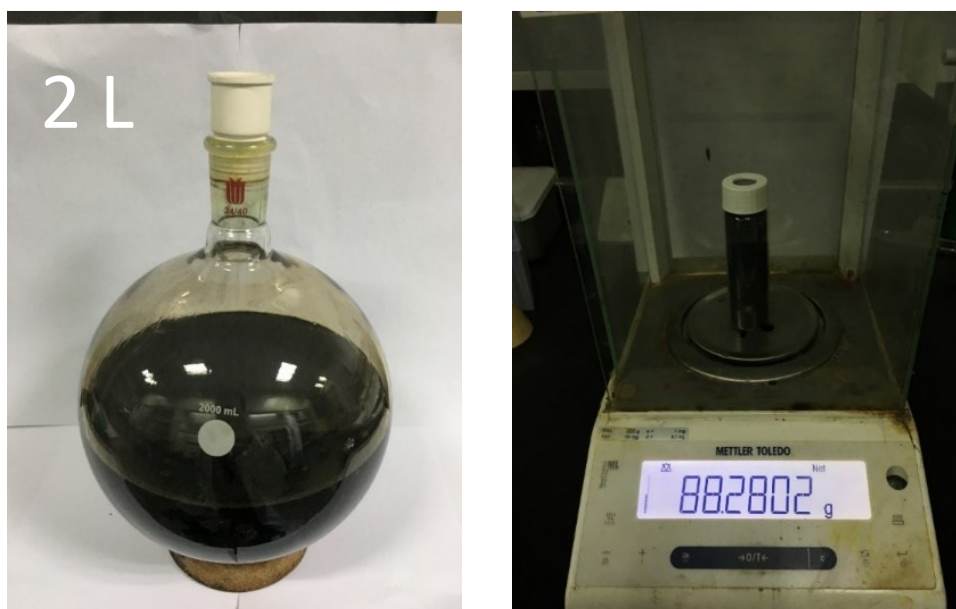
Supplementary Figure 6. Photos of scaled-up 2L synthesis. 88 g PbS-I NCs can be obtained in one-pot synthesis.
