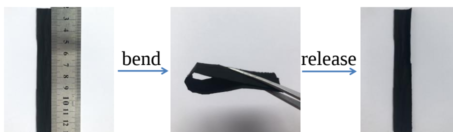
Supplementary Figure 2. Mechanical tests. Digital images of a piece of flexible NiSA/PCFM sample for 200 times bending tests.
