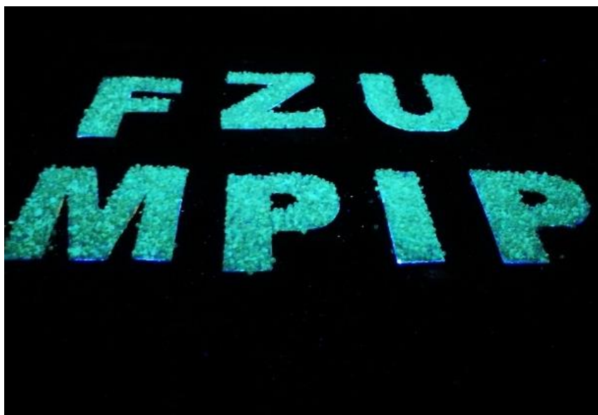
Supplementary Figure 22. Photo of UCN-coated glass beads pattern with words “FZU” and “MPIP” under the irradiation of UV light
