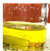
Supplementary Figure 1. Photos of SnI 2 sources and 0.9 M FA 0.75 MA 0.25 SnI 3 solutions with 10 mol% SnF 2 in DMSO using each SnI 2 source.
