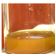
Supplementary Figure 1. Photos of SnI 2 sources and 0.9 M FA 0.75 MA 0.25 SnI 3 solutions with 10 mol% SnF 2 in DMSO using each SnI 2 source.
