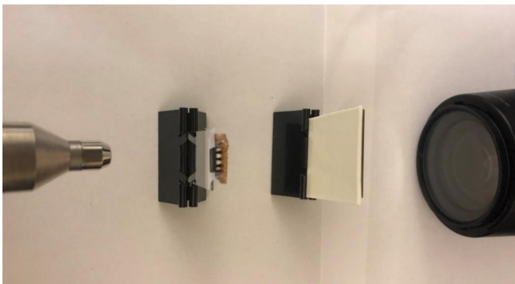
Supplementary Figure 9 | Projection configuration of a home-built X-ray imaging system.
