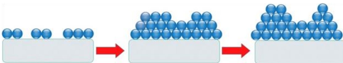
Supplementary Figure 1. Illustration of the suggested Stranski-Krastanov growth process of 3D Zn-Mn alloy.
