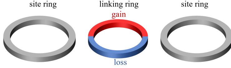
Fig. R4. Schematic for realizing asymmetric coupling in acoustics using ring resonators. Two acoustic ring resonators (site ring) are coupled through another ring (linking ring). Asymmetric coupling can be generated by putting gain and loss into the link ring.
